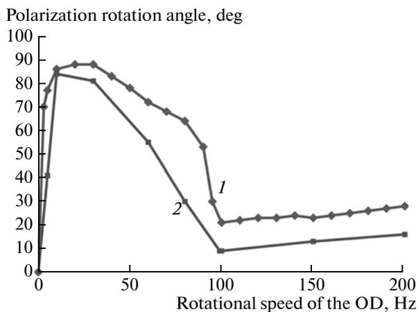
**Fig. 5.** Angle of rotation of polarization as a function of rotational speed of the OD for vertical (1) and horizontal (2) polarizations of the laser output.
