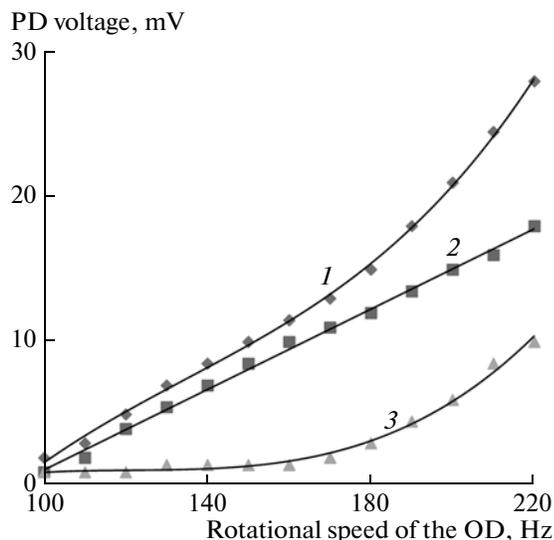
**Fig. 3.** Photodetector signal amplitude as a function of rotational speed of the OD for initial position of the polarizer (1), after polarizer rotation for minimum signal (2), and their difference (3).
