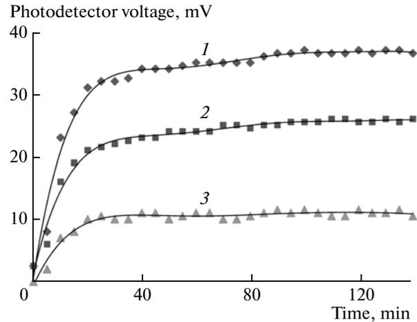
Fig. 4. Peak photodetector voltage amplitude as a function of time at a rotational speed of 150 Hz (1) for the initial position of the polarizer, (2) after polarizer rotation for the minimum signal, and (3) their difference.
