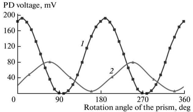
**Fig. 2.** Photodetector voltage as a function of angle of rotation of the polarizer for horizontal polarization of the laser output: (1) stationary OD, (2) at rotational speed of the OD equal to 80 Hz.
