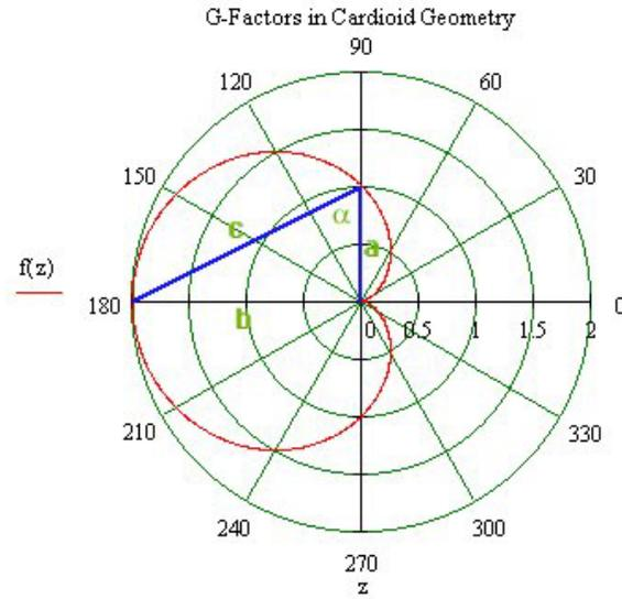
In figure 8, triangle side  $b$  is a unit length, equal to the radius of the sphere on which the cardioid path rests. As can be seen, side  $a$  is half the unit length and side  $c$  is the hypotenuse of right triangle  $\triangle abc$ .  $\triangle abc$  is a special form of right triangle where side  $b$  is twice side  $a$ , which we can call a Phi triangle (it is not a Golden triangle).
