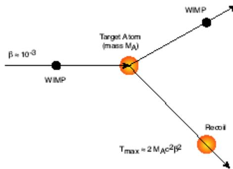
Fig.2. Model of interaction between WIMP – atom
