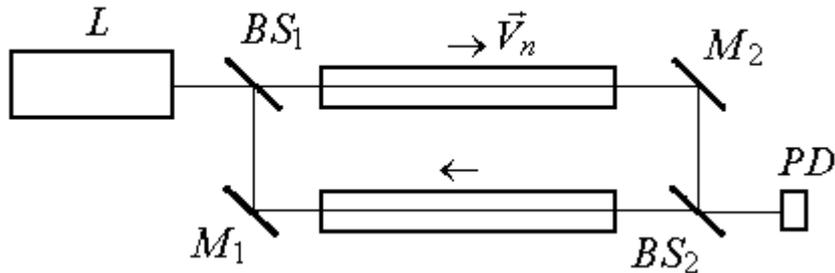
Fig.1. Fizeau-type interferometer with the one-passage scheme for laser beams.
