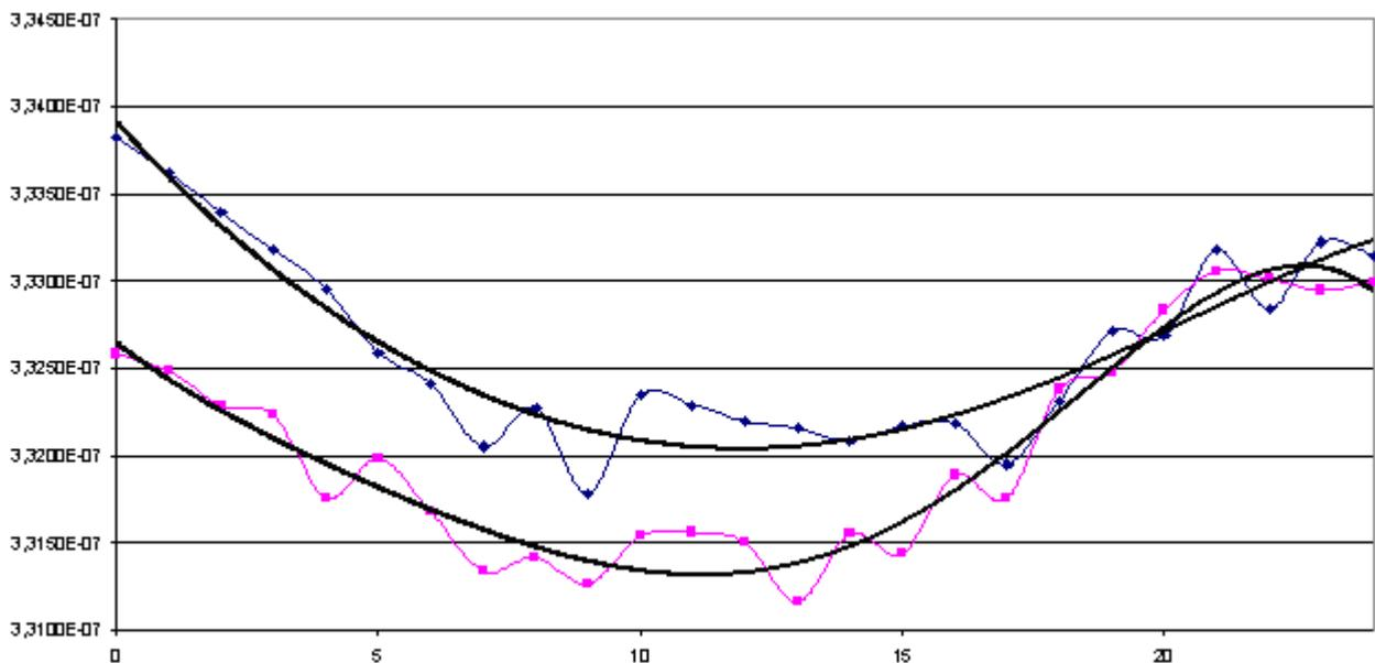
Fig.5. Dependence of signal on turn angle of the interferometer for direct and reverse rotations. Unit of axis  $x$  is equal to 15 degrees. Dark curves are as a result of spline - interpolation.
