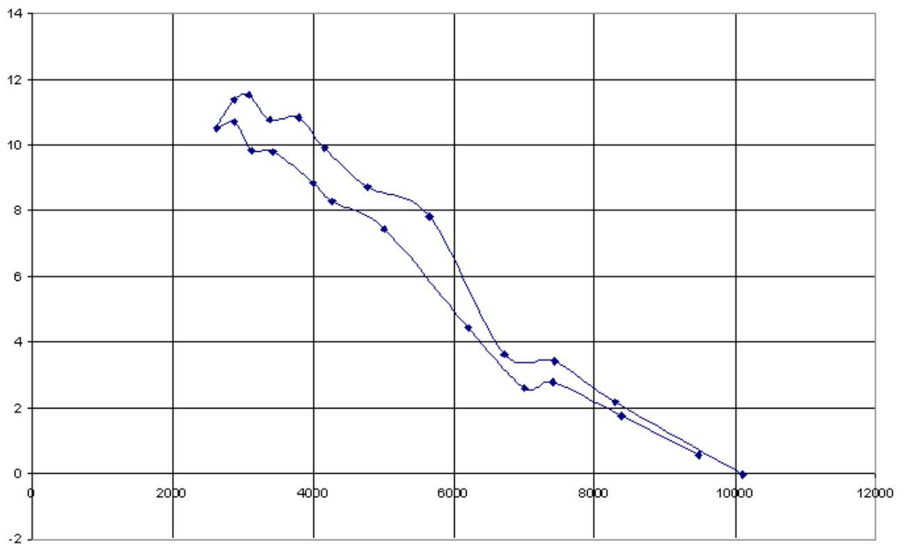
Fig.4. Dependence of relative difference between calculated IP shift without Fizeau's effect and measured IP shift (%) on rotation period (mks).
