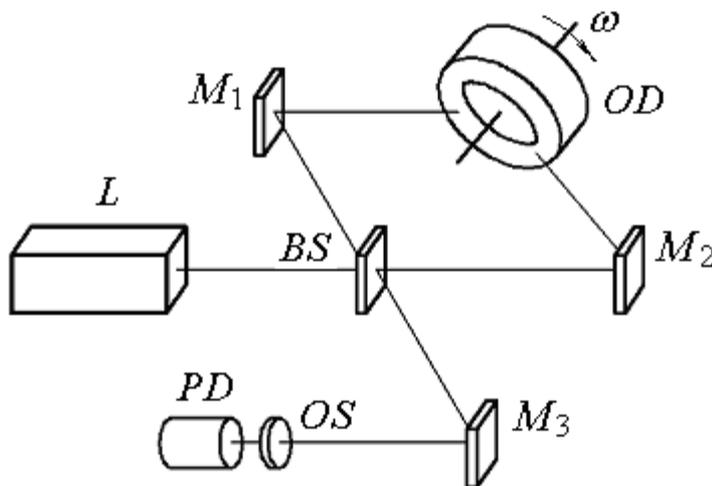
Fig.2. Two-beams one-passage interferometer with rotating OD.
